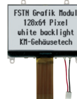
white backlight KM Grafik LCD 128 x 64
